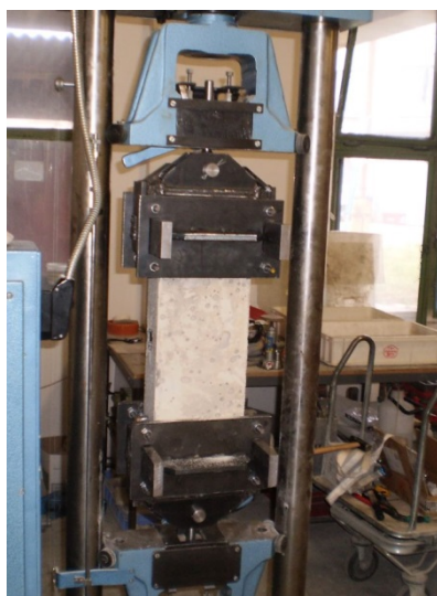
Figure 8 – Detail of a tensile strength testing rig
