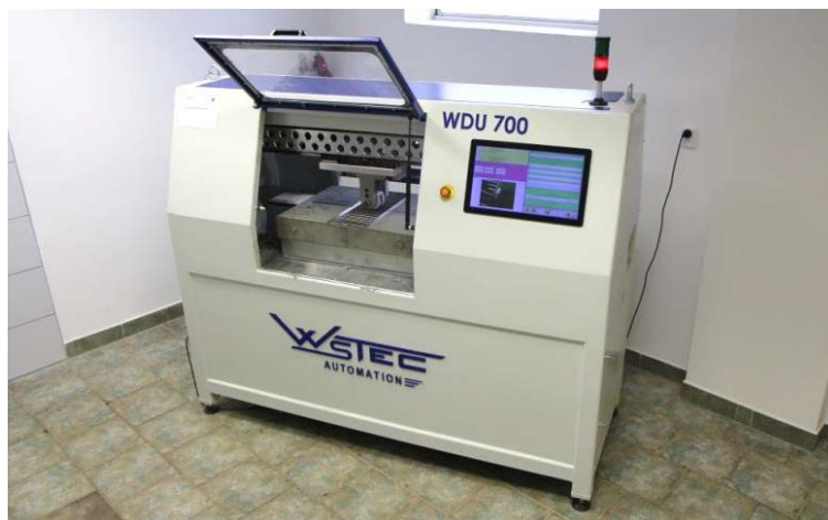
Figure 5 – WSTEC rig developed for mechanical exposure testing
